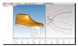
This provides the best way to ensure proportions of the shoe are accurate and provides technical CAD data to manufacturers that requires no interpretation.
