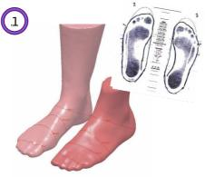
Multiple 3D views & 2D sections allow simple evaluation of last & foot shapes
